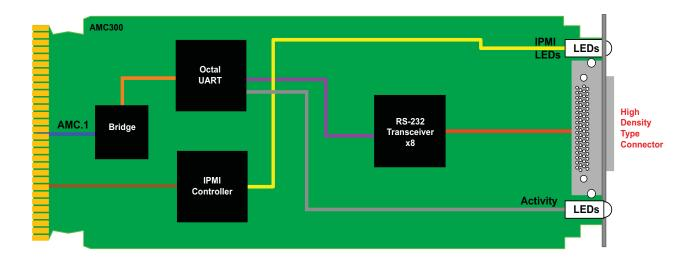
FIGURE 1. AMC300 Functional Block Diagram
