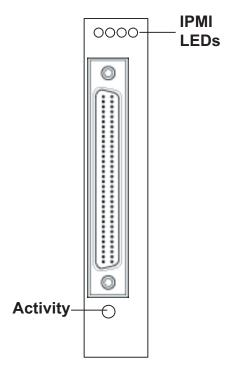
FIGURE 2. AMC300 Front Panel
